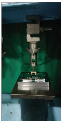
**Figure 1:** Universal testing machine checking the strength of the material
