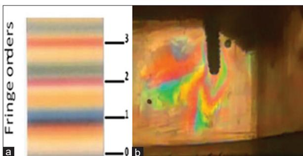
Figure 3: (a and b) Relation between stress level and fringe order used
