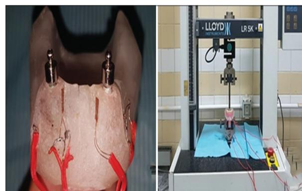
**Figure 2:** A – strain gauges fixed mesial and distal to the implants B – universal testing machine applying load on implant overdenture
