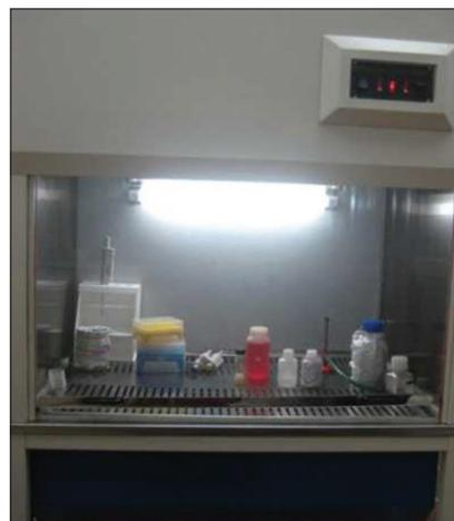
Figure 1: Vertical laminar air flow unit
