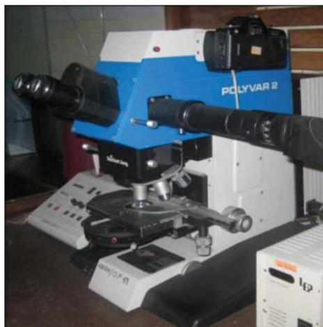
**Figure 3:** Compound microscope with attached camera with macro zoom
